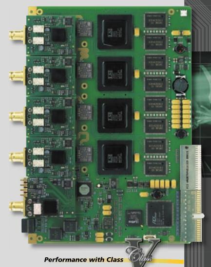
The DC Series Digitizers use large-scale integrated circuit technology to reduce size and power requirements. This essential technology allows the DC211, DC241 and DC271 to deliver the fastest sampling rate, highest bandwith and most memory for any digitizer in a 6 U Compact PCI/PXI package.
