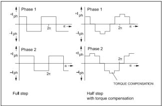
The figure shows the phase currents for the full step mode and those of the half step mode with torque compensation.
