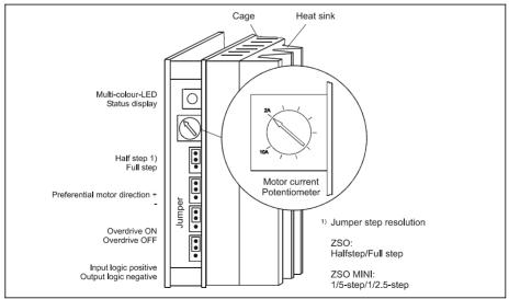
Fig. 19: Front view - front panel removed (ZSO 102-140 to 182-140)
