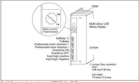
Fig. 18: Front view - front panel removed (ZSO 22-40 to 92-70)
