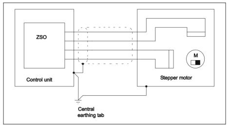
Fig. 12: Motor lead shielding
