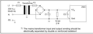
Fig. 13: Example of supply unit
