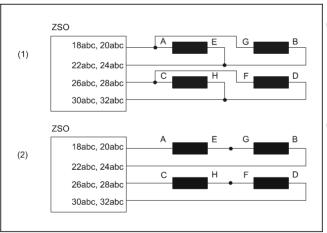
8-lead stepper motor connected as a 4-lead stepper motor
