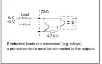
Rated current = 20 mA U<sub>max</sub> = 30 V U<sub>CE sat</sub> at 20 mA < 1 V
