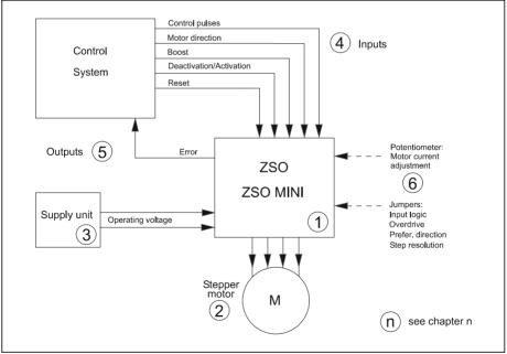
Fig. 1: Connecting diagramm for ZSO power stages
