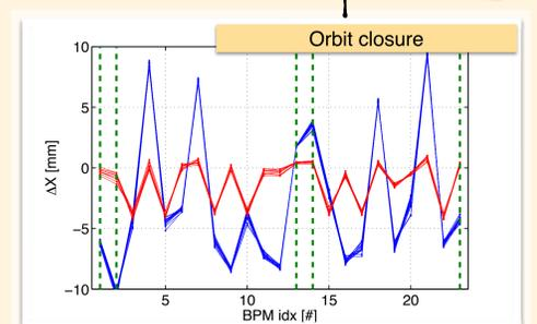
Horizontal beam profile at the end of the linac in a dispersive BPM for different single shots. The blue lines are before energy flattening correction, the red lines after the correction.
