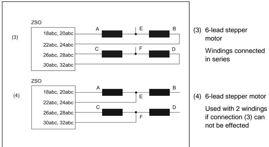
Fig. 10: 6-lead motor connection
