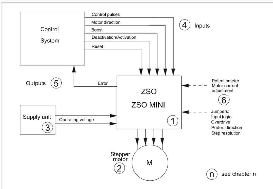
Fig. 1: Connecting diagram for ZSO power stages
