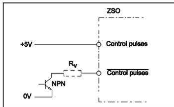
Fig. 15: Input connection NPN-transistor
