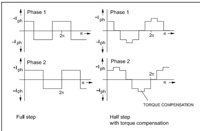
Fig. 6: Phase currents in the full step and the half step mode
