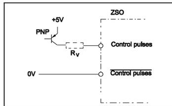
Fig. 16: Input connection PNP-transistor
