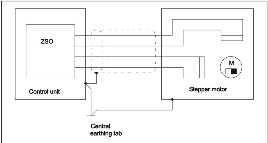
Fig. 12: Motor lead shielding
