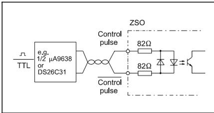
Fig. 14: Push-pull input connection
