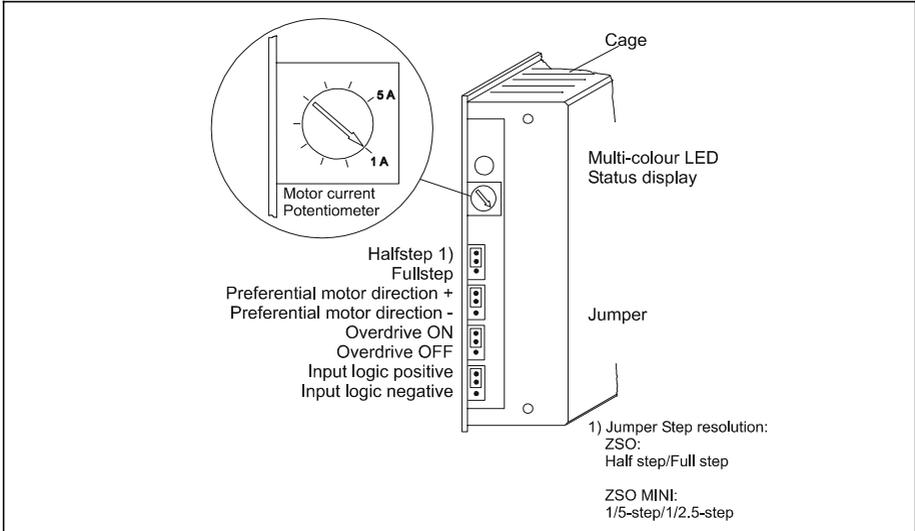
Fig. 18: Front view - front panel removed (ZSO 22-40 to 92-70)
