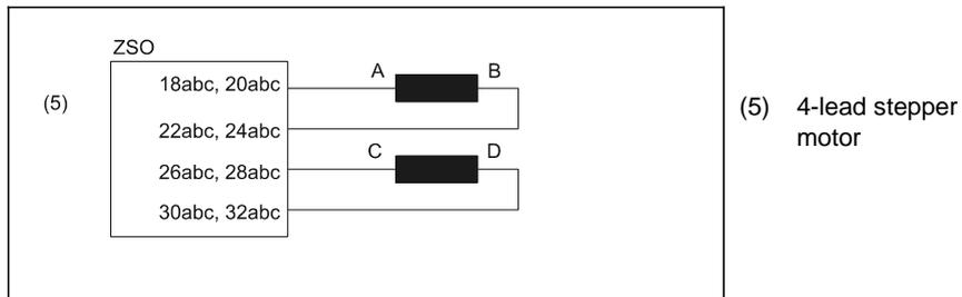
Fig. 11: 4-lead motor connection
