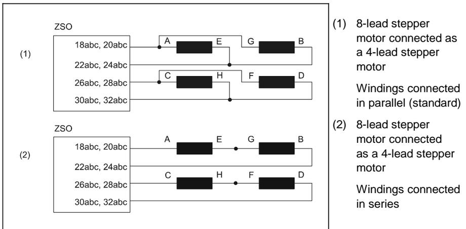
Fig. 9: 8-lead motor connection
