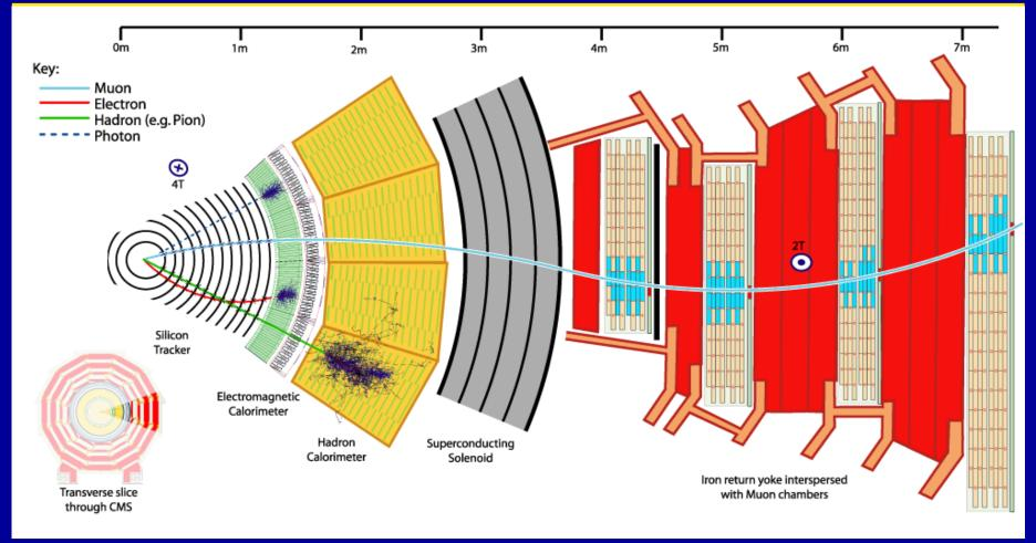
Deflection ~ BL2/p → need high B (superconducting) and large magnets
